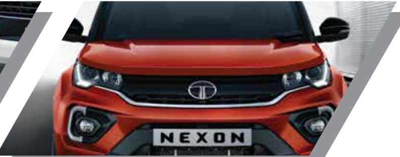
AUTOMATIC HEADLAMPS Light up automatically in dark conditions.
